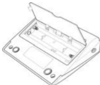
2. Place the batteries (4 "AA" Alkaline batteries) in the
